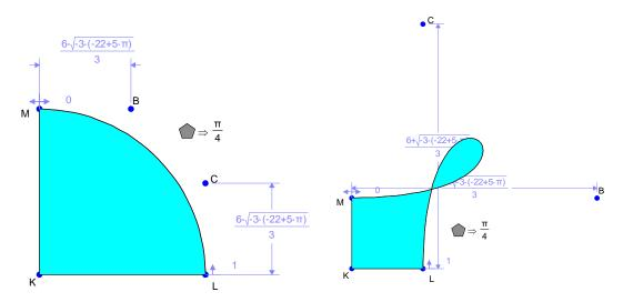
Figure 10: two solutions yielding the same area under the spline. Only one is a good approximation for the quarter circle!
